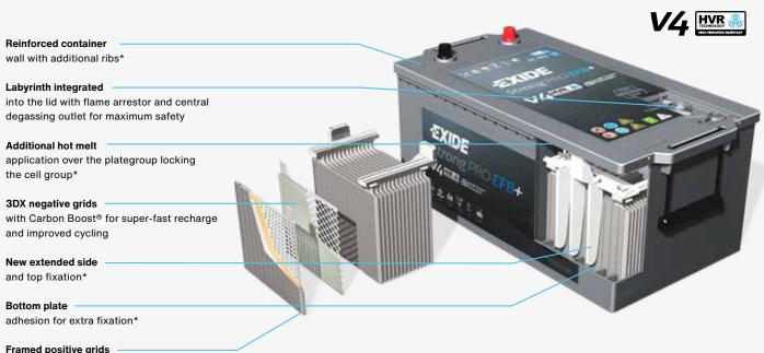
with heavy-duty polyethylene separator and glass mat for homogeneous compression
