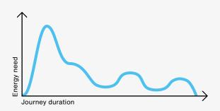
Batteries in this category cover twice the supply needs of a boat. They are used for starting the engine as well as for the operation of other electrical devices. These batteries are characterized by high peaks of power and variable power drain, which causes the battery to discharge during the journey. The electrical unit used to measure dual supply need is Wh\*.
